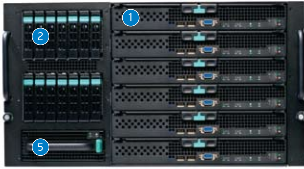
Figure 1. Intel® Modular Server integrates multiple levels of infrastructure in a single chassis:
